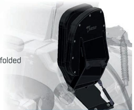
The entire Fendt cab was scanned in 3D in order to develop the best technical solution for a high-quality passenger seat. The pleasantly rounded cushion contour evolved after evaluating various samples.
